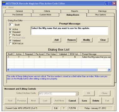
The next step is to set the Action Code to scan an alternate field, if the system does not find an asset number. If we enter a Manufacturer instead, the system will not find that entry in the asset number field, and will scan the Manufacture Field (I4202) instead. The selection is shown at right.
